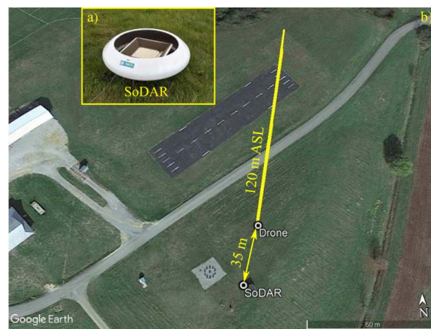
Fig. 4 (a) A close-up image of the SoDAR wind velocity profiler used to validate multirotor sUAS wind profiles. (b) A schematic of the experiment setup used at Virginia Tech Kentland Experimental Aerial Systems Laboratory on June, 29th, 2020 to validate multirotor sUAS wind velocity profiles next to SoDAR wind profiler.
