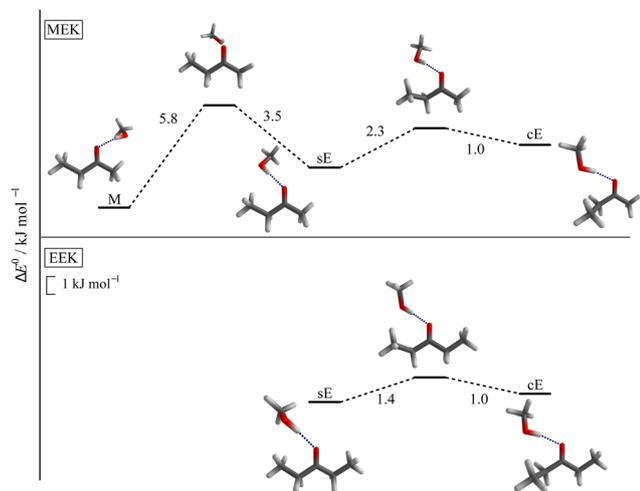
**Fig. 3** Most stable conformers for MEK (upper panel) and EEK (lower panel) solvated by MeOH and the relevant transition states for the interconversion, calculated at B3LYP-D3(BJ,ABC)/def2-TZVP level. The *syn*-ethyl- or sE-sided and clinal-ethyl- or cE-sided structure motifs are predicted for both ketones. For the methyl- or M-sided MEK complex only the most stable *syn*-conformation is shown (see also ESI<sup>†</sup> Fig. S4 and Table S4).
