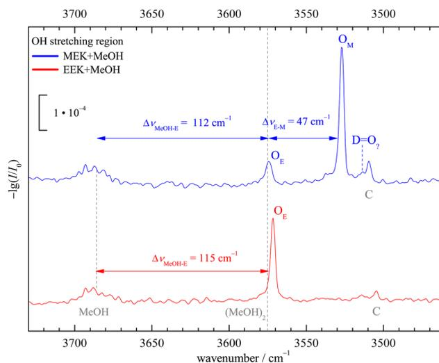
**Fig. 4** Jet FTIR OH-stretching spectra of MeOH in co-expansion with MEK and EEK including the MeOH monomer region. C marks a non 1:1 stoichiometry and D=O<sub>2</sub> is the largest isolated signal which might perhaps be attributed to a third 1:1 isomer in the MEK case, beyond the dominant O<sub>M</sub> (M docking) and the secondary signal O<sub>E</sub> (sE docking, common to both ketones). For details, see the main text.
