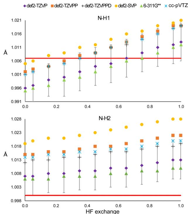
Fig. 5 N–H1 (top) and N–H2 (bottom) distances obtained from the HAR, using different basis sets with the PBE<sub>x</sub> functional. The red line corresponds to the neutron diffraction value.
