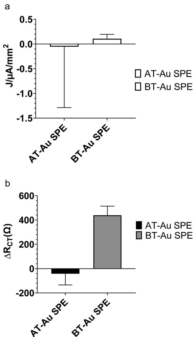
Fig. 4 Comparison of performance of AT-Au and BT-Au SPEs, following MIP modification and protein (1 nM) rebinding. Effect on (a) CV peak anodic current change ( $J$  in  $\mu\text{A}/\text{mm}^2$ ) and (b) charge transfer resistance ( $R_{CT}$  in  $\Omega$ ) change. Data represents mean  $\pm$  S.E.M.,  $n = 3$ .
