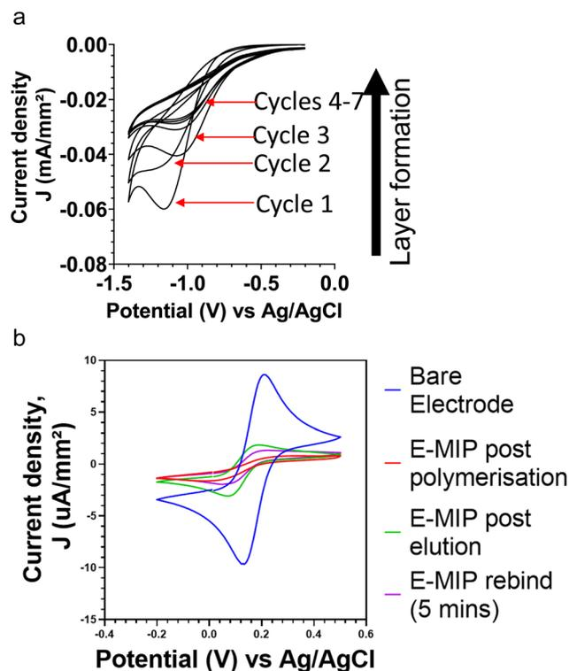
**Fig. 1** (a) Layer by layer deposition of pNHMA E-MIP on BT-Au SPE vs. Ag/AgCl reference electrode using cyclic voltammetry (–0.2 V and –1.4 V vs. Ag/AgCl reference; 7 cycles at 50 mV s<sup>-1</sup>). (b) CV of ferrocyanide redox marker at different stages of electrode modification: bare (blue); post E-MIP polymerisation (red); post template, BHB elution (green); and after 5 min of template, BHB (1 nM) rebinding (purple).
