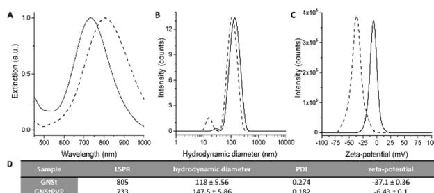
**Fig. 1** (A) UV-Vis-NIR extinction spectra, (B) hydrodynamic diameters determined by dynamic light scattering measurements, and (C) zeta-potential of colloidal GNSts (dashed line) and GNStsPVP (full line). (D) Table summarizing the physicochemical characteristics of the colloidal suspensions.
