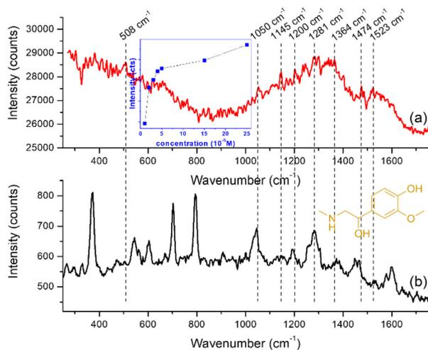
**Fig. 6** (a) The SERS spectrum of metanephrine on the GNStsPVP film at  $10^{-5}$  M concentration; dependence of the SERS signal on metanephrine concentration is displayed in the inset. (b) Raman spectrum of metanephrine at  $5 \times 10^{-2}$  M concentration. Both spectra were obtained using 785 nm laser excitation.
