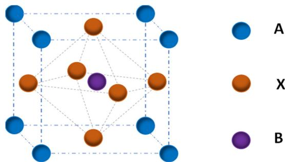
Fig. 9 The perovskite crystal structure having a general formula of ABX<sub>3</sub>.
