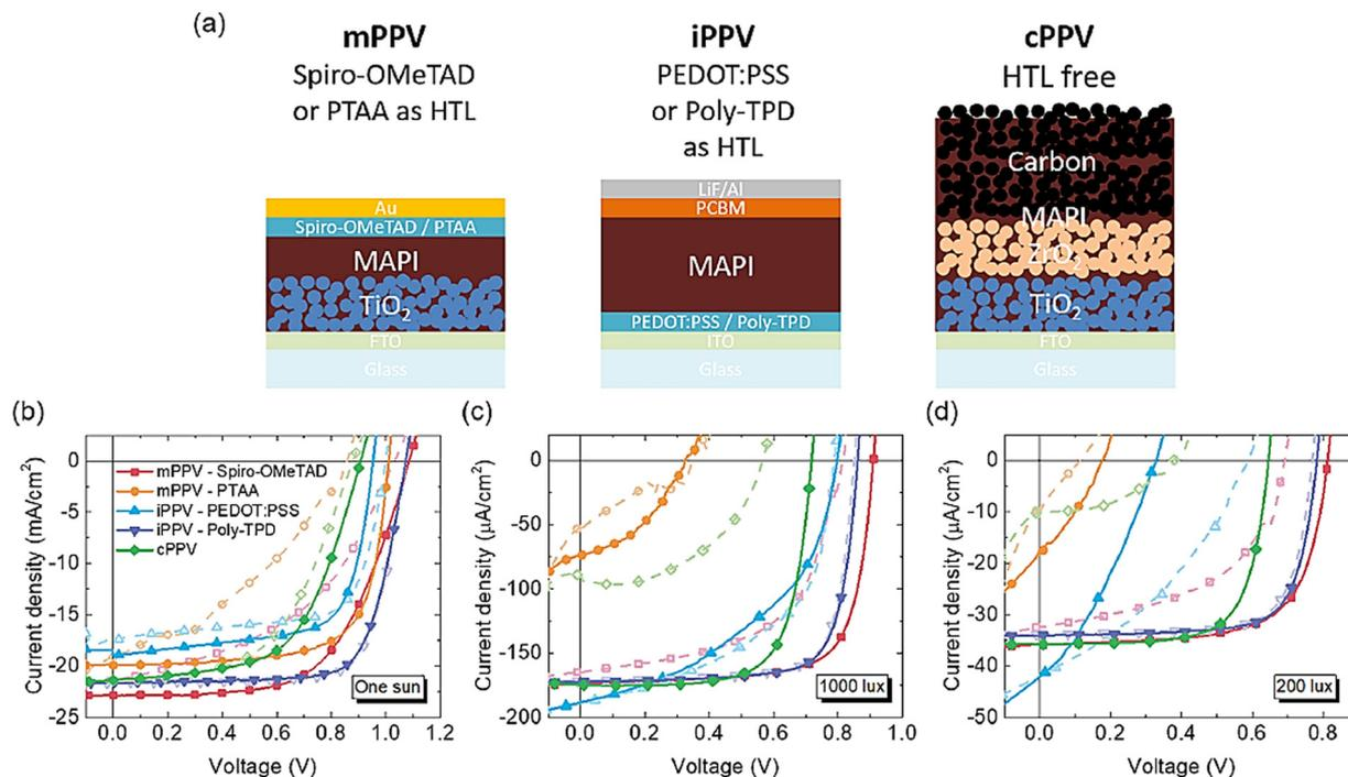
**Fig. 10** (a) Schematic of three kinds of device architecture (mesoporous PSC: mPPV, inverted PSC: iPPV, HTL free-carbon based: cPPV) with different HTLs. Forward and reverse  $J-V$  characteristics of five different device configurations under (b) 1 sun, (c) 1000 lux FL illumination, and (d) 200 lux FL illumination. Reproduced from ref. 191 with permission from [Wiley], copyright [2019].
