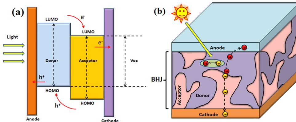
Fig. 5 Schematic of the working principle of (a) the two-layer donor-acceptor heterojunction, (b) a bulk heterojunction-based organic solar cell.
