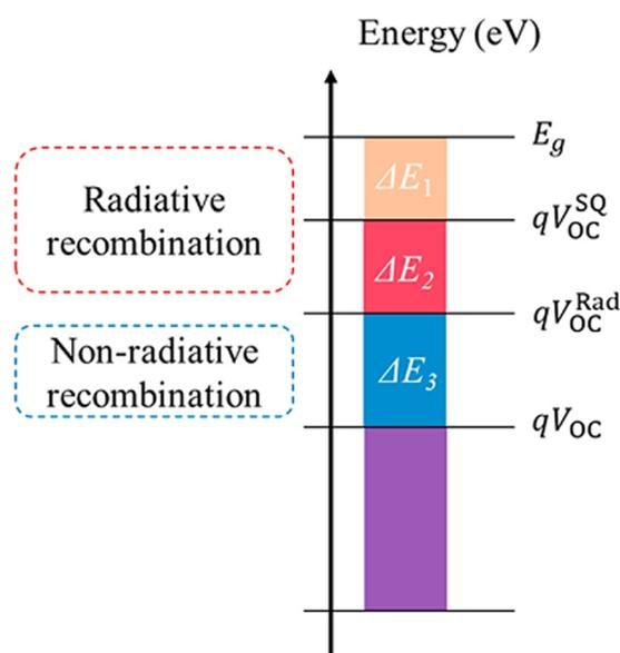
Fig. 2 Combination of losses in open circuit voltage from the bandgap energy ( $E_g$ ) due to radiative and non-radiative recombination.  $V_{OC}^{SQ}$  is the voltage at the maximum Shockley–Queisser limit and  $V_{OC}^{Rad}$  is the open circuit voltage under radiative recombination. Reproduced from ref. 48 with permission from [ACS], copyright [2020].
