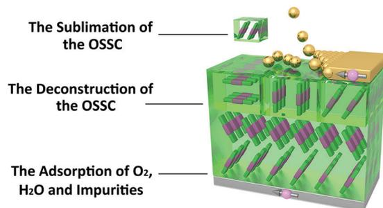
**Fig. 2** A schematic diagram of a vertical spin valve device based on an OSSC, which shows the great challenges related to device fabrication. These include the sublimation and deconstruction of the OSSC because of high heat and kinetic energy during the deposition of the top electrode, and the adsorption of  $O_2$ ,  $H_2O$ , and impurities at the surface of the bottom electrode, which will destroy efficient spin injection at the bottom interface.
