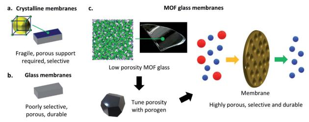
Fig. 6 Schematic of the drawbacks and advantages of (a) crystalline membranes and (b) glass membranes, and (c) the formation of new MOF glass membranes by the introduction of significant porosity into MOF glasses.
