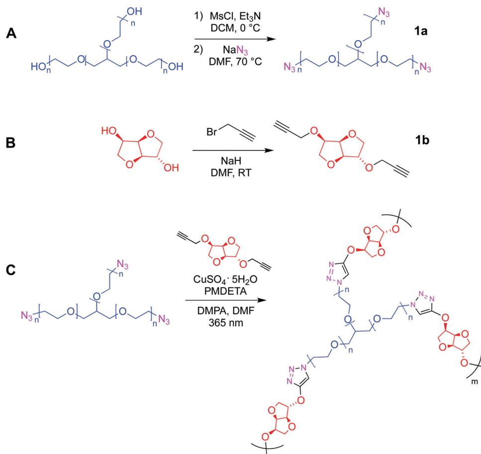
**Scheme 1** Synthetic protocols employed in the preparation of (A) triazide glycerol ethoxylate and (B) bis-alkyne isosorbide derivatives. (C) Synthesis of hydrogel films via Cu(I) mediated photo-click reaction.
