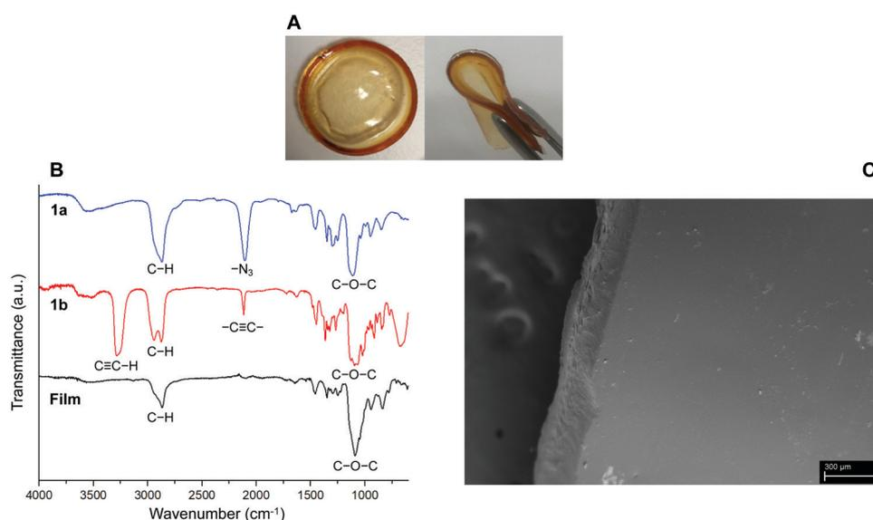
Fig. 1 (A) Digital images of obtained flexible hydrogel films (diameter of circular film = 4 cm). (B) FTIR spectra of **1a**, **1b** and the film. (C) SEM image of the hydrogel film. Scale bar = 300 μm.
