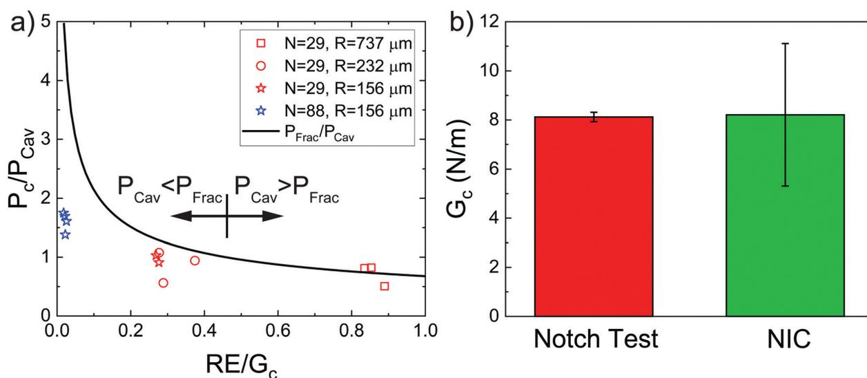
Fig. 4 (a) Plot of the experimentally observed critical expansion pressure  $P_c$  normalized by  $P_{\text{Cav}}$  against  $RE/G_c$ . The black line represents the point at which fracture is predicted to occur. (b) Plot showing the comparison between  $G_c$  measured with notch tests by Barney *et al.*<sup>16</sup> and measured with NIC in this work when  $RE/G_c \approx 0.84$ .
