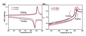
Fig. 3 Phase transitions of R-CSAI and S-CSAI. (a) DSC curves in a heating-cooling run. (b) Temperature-dependent  $\varepsilon'$  at 1 MHz upon heating and cooling.
