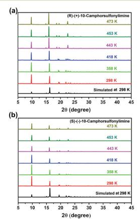
**Fig. 4** Phase transitions of *R*-CSAI and *S*-CSAI. (a) Variable-temperature PXRD patterns of *R*-CSAI. (b) Variable-temperature PXRD patterns of *S*-CSAI.
