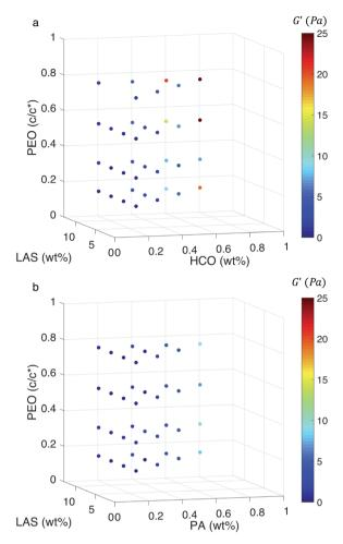
Fig. 6 Bulk rheological measurements for varying concentrations of (a) HCO and (b) PA colloidal rod systems. The three axes are the concentration of each component and the color of the data indicates the value of the storage modulus, G'. Warm colors are the maximum measured storage moduli, which indicates higher elasticity of the material. Cool colors represent minimum storage moduli, which indicates low to no elasticity of the material.
