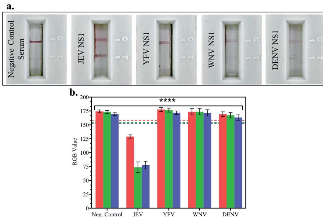
Fig. 5 Specificity studies of the fabricated LFA against other cross-reactive flaviviral NS1 Ags: (a) LFA strip images of testing 1  $\mu$ g ml<sup>-1</sup> NS1 Ag of different *Flaviviruses* spiked in JEV negative serum; (b) bar graph of the RGB values of LFA cross-reactive test strips using the smartphone colorimeter application compared to the RGB lines of the LOD (10 pg ml<sup>-1</sup>) as the positive control.
