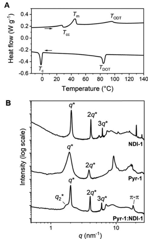
Fig. 1 (A) DSC trace (second heating and cooling cycle) of **Pyr-1:NDI-1**. A temperature ramp of 10 K min<sup>-1</sup> was used. Endothermic heat flows have a positive value. (B) 1D transmission scattering profiles of **Pyr-1:NDI-1** (bottom), **Pyr-1** (middle) and **NDI-1** (top) at room temperature.
