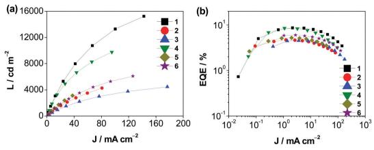
Fig. 7 (a) J-L curves and (b) EQEs vs. current density of the solution-processed devices based on **1–6**
