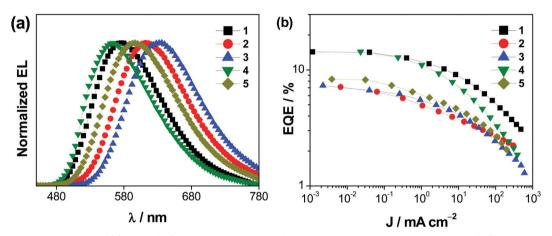
(a) Normalized EL spectra and (b) plots of EQEs vs. current density of the vacuum-deposited devices based on 1-5.
