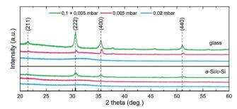
Fig. 1 Grazing incidence XRD spectra of ITO deposited following the LP (0.005 mbar); LP with buffer (0.1  $\pm$  0.005 mbar) and high pressure (0.02 mbar) conditions on glass (top) a-Si:H-coated c-Si substrates (bottom), all annealed at 200 °C in air.
