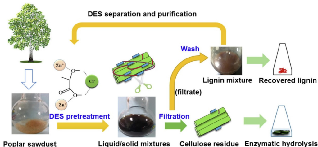
Fig. 2 Schematic representation of the DESs pre-treatment process. Reprinted with permission from ref. 58. Copyright 2022, Elsevier.
