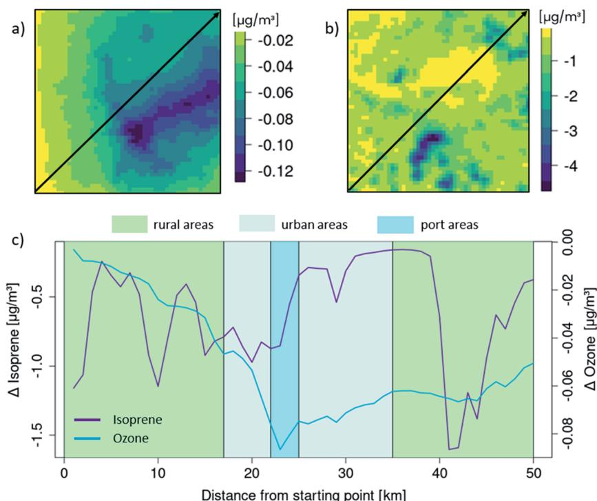
Fig. 10 Absolute differences in ozone concentrations (10a) and isoprene concentrations (10b) due to drought stress in July 2018 and diagonal transect (SW-NE) of differences in ozone and isoprene concentrations (10c) due to drought stress throughout the study domain for a dry period in July 2018.
