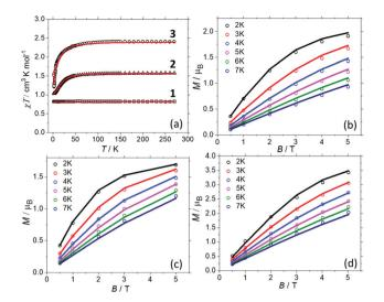
Fig. 2 (a) Magnetic susceptibility data for 1-3 measured in an applied field, B = 0.1 T. (b-d) Magnetisation data for 1-3, respectively, in the T =2-7 K range in fields up to, B=5 T. The solid lines represent the simultaneous fits of the susceptibility and magnetisation data to spin-Hamiltonian (1). See the main text and Table 1 for the best fit parameters
