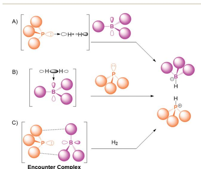
**Scheme 1** Mechanisms for the splitting of H<sub>2</sub> by an FLP comprising a bulky phosphine and borane as alternatives to true termolecular reactivity. A: pre-association of the phosphine and H<sub>2</sub>; B: pre-association of the borane and H<sub>2</sub>; and C: pre-association of the phosphine and borane as an encounter complex.
