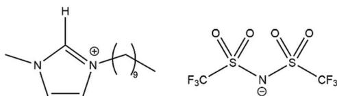
Fig. 5 Structure of ionic liquid [C<sub>10</sub>mim][NTf<sub>2</sub>].
