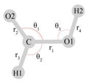
Fig. 2 Valence coordinates defined by Richter and Carbonniére<sup>56</sup> and adopted in ref. 2, 30, 53 and 79 for the monomeric formic acid molecule. The torsional coordinates  $\tau_1$  and  $\tau_2$  (not depicted) describe the out-ofplane motions of H1 and H2, respectively. Reprinted with permission from ref. 56 from AIP Publishing, copyright 2018.
