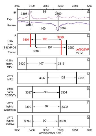
Fig. 4 Comparison of experimental OH stretching band positions (from Fig. 2, trace c, IR and Fig. 3, trace c, Raman) and their splitting with harmonic and anharmonic predictions for the (TgF) dimer. See text for explanations
