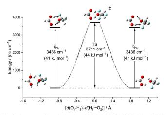
Fig. 6 Energy profile calculated at B3LYP-D3(BJ)/def2QZVP level (ZPE corrected) for the proton exchange promoted by the symmetric OH stretch vibration in the most stable (T<sup>g</sup><sub>q</sub>F) dimer. As the exchange coordinate, the difference between the chemical and the hydrogen-bonded distances of the two jumping protons from the acid oxygens is chosen. The transition state (1620i cm $^{-1}$ ), where this difference vanishes, has  $C_s$
