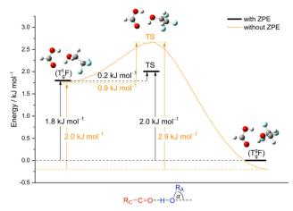
Fig. 5 Energy profile calculated at B3LYP-D3(BJ)/def2QZVP level for the isomerism of the metastable (T<sub>q</sub><sup>t</sup>F) complex on the left to the global minimum (T<sub>a</sub><sup>g</sup>F) structure on the right (lone pair switch) along the hinge angle. Shown with and without zero-point vibrational energy.
