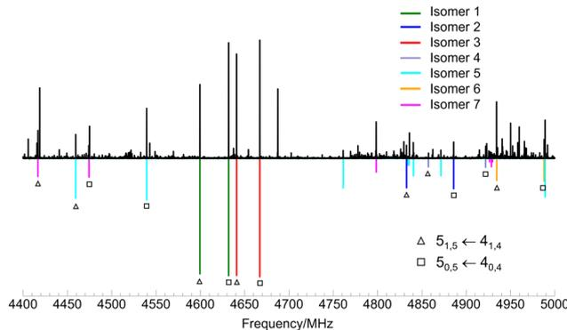
Fig. 2 Section of the rotational spectrum of limonene–(H<sub>2</sub>O)<sub>2</sub> predicted at a rotational temperature of 1 K, showing the 5<sub>0,5</sub> ← 4<sub>0,4</sub> and 5<sub>1,5</sub> ← 4<sub>1,4</sub> rotational transitions for all observed isomers. Upper trace shows the experimental spectrum, lower trace shows the simulated spectrum using the experimentally determined rotational constants.
