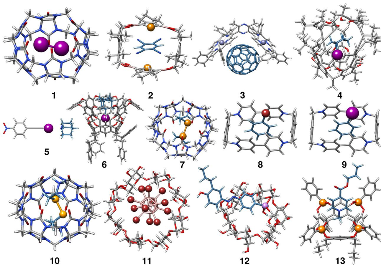
Fig. 1  $r^2$ SCAN-3c[SMD] optimized geometries of the 13 host-guest complexes of the HS13L benchmark set. For better visibility, the C and H atoms of the guest molecules are colored in blue and light blue, respectively.
