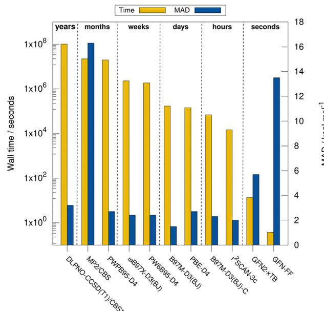
Fig. 4 Computational wall times (Intel<sup>®</sup> Xeon<sup>®</sup> E5-2660 v4 @ 2.00 GHz CPU) for the best performing methods of the assessed levels of theory for the calculation of the association energy of complex **6** in combination with the respective MADs to the “back-corrected” experimental values for the HS13L-CI. Complex **3** is not included in the MAD of “DLPNO-CCSD(T1)/CBS” indicated by the \*.
