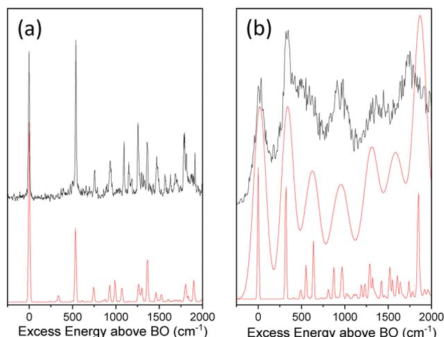
**Fig. 5** Comparison between the experimental and FC simulations of (a) the  $D_0$ – $D_4$  transition of  $C_1^{\bullet+}$  and (b) the  $D_0$ – $D_3$  transition of  $C_4^{\bullet+}$ . Calculated frequencies (UCAM-B3LYP/aug-cc-pVDZ) scaled by 0.95. BO is for “Band Origin”.
