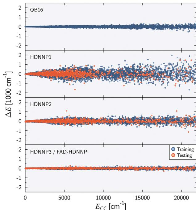
Fig. 2 Energy difference  $\Delta E = E_{CC} - E_{PES}$  as a function of the reference energy  $E_{CC}$  relative to the energy of the global minimum for the QB16 PES,<sup>55</sup> HDNNP1, HDNNP2, and HDNNP3 (=FAD-HDNNP). The root-mean-squared errors (RMSE) for the HDNNPs are provided in Table 1.
