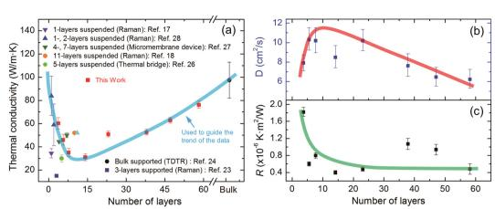
Fig. 7 (a) In-plane thermal conductivity, (b) hot carrier diffusion coefficient, and (c) interface thermal resistance of multiple MoS<sub>2</sub> films as a function of the film's number of layers. Reproduced from ref. 35 with permission from the PCCP Owner Societies, copyright 2018.
