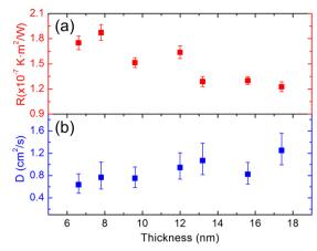
Fig. 6 (a) Interface thermal resistance, and (b) hot carrier diffusion coefficient of seven MoS<sub>2</sub> nm-thick films supported on c-Si. Reproduced from ref. 7 with permission from American Chemical Society, copyright 2017.
