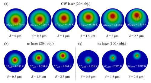
Fig. 10 Results of numerical analysis conducted by Zobeiri et al. to investigate the effect of laser spot position on the uncertainty of measured D of a suspended WS<sub>2</sub> film. (a) CW laser heating ( $20 \times$ ), (b) ns laser heating ( $20 \times$ ), and (c) ns laser heating ( $100 \times$ ). Reproduced from ref. 34 with permission from Elsevier, copyright 2019.
