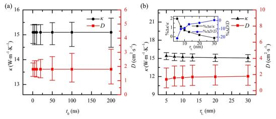
Fig. 8 Effects of (a) laser pulse width and (b) laser absorption depth on the uncertainty of measured *D* (right vertical axis of both plots). Reproduced from ref. 34 with permission from Elsevier, copyright 2019.
