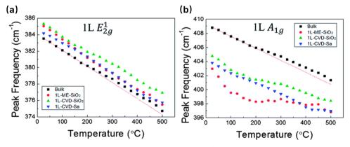
Fig. 3 Temperature dependence of the two Raman modes of monolayer  $MoS_2$ : (a)  $E_{2g}^1$  and (b)  $A_{1g}$ . Reproduced from ref. 30 with permission from the Royal Society of Chemistry, copyright 2014.
