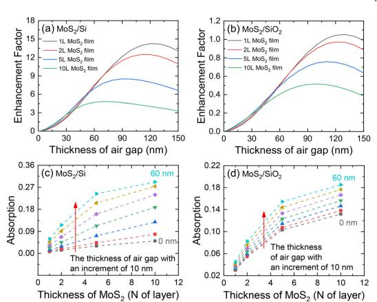
Fig. 2 Laser absorption in supported MoS<sub>2</sub> films. Absorption enhancement factor in the MoS<sub>2</sub> layer of (a) MoS<sub>2</sub>/Si sample and (b) MoS<sub>2</sub>/SiO<sub>2</sub> sample against the air gap thickness. Absolute laser absorption in the MoS<sub>2</sub> layer of (c) MoS<sub>2</sub>/Si sample and (d) MoS<sub>2</sub>/SiO<sub>2</sub> sample against MoS<sub>2</sub> thickness.
