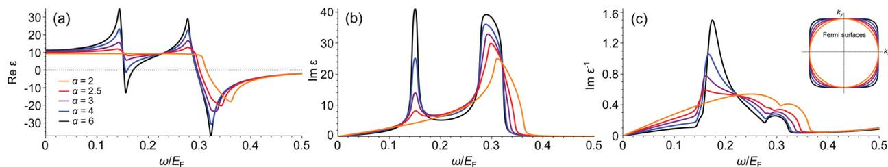
**Fig. 5** (a) The real and (b) the imaginary parts of the dielectric function and (c) the loss function of an electron system with the square symmetry evaluated at  $\mathbf{q} = (0.15\sqrt{E_F}, 0.075\sqrt{E_F})$  for different anisotropic factors  $\alpha$ . The Fermi surfaces corresponding to each value of  $\alpha$  are sketched in the inset of (c).
