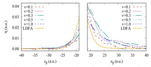
Fig. 7 Friction coefficient for the antiproton moving in vacuum outside the Na<sub>106</sub> cluster. The in-going (left panel) and out-going (right panel) trajectory segments are shown. Different curves correspond to the results obtained for different antiproton velocities  $\nu$  as indicated in the insert, where  $\nu$  is given in atomic units. The orange curve denoted as "LDFA" shows the friction coefficient calculated within the LDFA approximation
