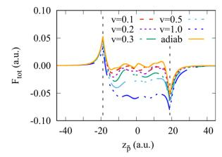
Fig. 2 Total force acting on the antiproton crossing the Na<sub>106</sub> clusters. Different curves correspond to the results obtained for different antiproton velocities  $\nu$  as indicated in the insert, where  $\nu$  is given in atomic units. The orange curve denoted as "adiab" shows the adiabatic result. Vertical dashed lines indicate the border of the positive background of the jellium
