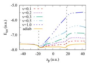
Fig. 1 Total energy of the Na<sub>106</sub> cluster as a function of the antiproton position. Different curves correspond to the results obtained for different antiproton velocities  $\nu$  as indicated in the insert, where  $\nu$  is given in atomic units. The orange curve denoted as "adiab" shows the adiabatic result. Vertical dashed lines indicate the border of the positive background of the iellium cluster
