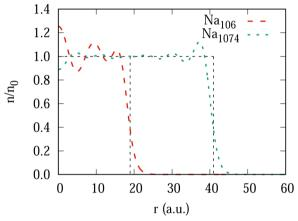
Fig. 9 Ground state electron density profile of the spherical clusters  $Na_{106}$  and  $Na_{1074}$  in the units of the constant background density  $n_0$  (thin dashed line) as a function of the radial coordinate
