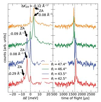
Fig. 3 Examples of time of flight measurements (right) and their conversion to energy exchange between the helium atoms and the bilayer (left). Arrow annotations indicate identified ZA-mode peaks in the left panel. Annotations next to the ZA-peaks gives their corresponding  $\Delta K$ -value. Scattering angles are given in descending order, with the first angle corresponding to the upper spectrum. The intensity of the spectra have been arbitrarily shifted to increase visibility.
