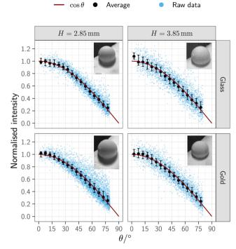
Fig. 5 Extracted scattering distributions from the 100 μm sphere both with and without gold coating, with insets showing the SHeM images the data was extracted from. The data is normalised by removing the background then scaled so that the fitted cosine has an amplitude of unity. It is clear that the atoms are scattered in a broad diffuse distribution with a stronger tendency for scattering close to the surface normal
