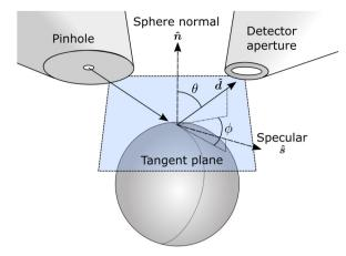
Fig. 3 Co-ordinate system and vectors used in the derivation of the relation between image positions and incidence and detection angles. d is the vector towards the detector,  $\hat{\boldsymbol{n}}$  is the unit normal to the sphere at the beam-sphere intersection point and  $\hat{\mathbf{s}}$  is the vector pointing in the specular reflection direction.
