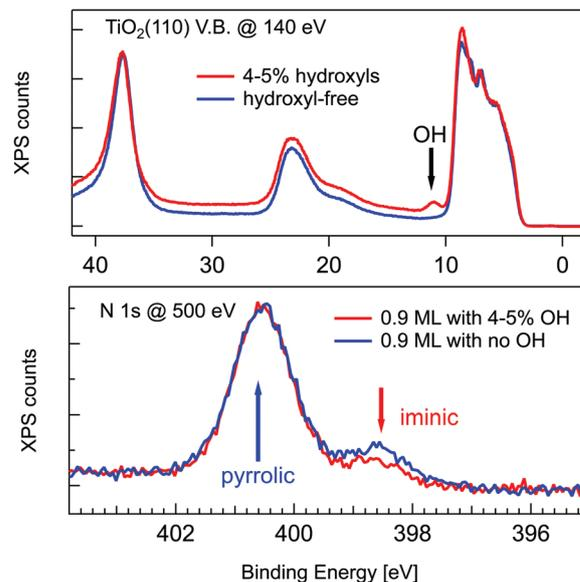
Fig. 4 Upper panel: Valence band photoemission from a slightly hydroxylated (red line) and a hydroxyl-free surface (blue line) before deposition; the OH  $3\sigma$  peak is marked with an arrow. Lower panel: Photoemission spectra of the N 1s peak for 0.9 ML of 2H-TPP deposited at RT on the same surfaces of the upper panel. Reproduced from ref. 47 with permission from the American Chemical Society, Copyright 2017.
