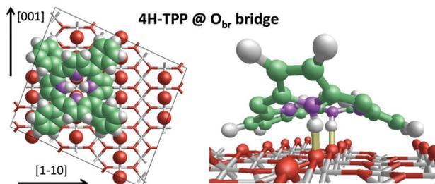
Fig. 5 Left: Top view of the 4H-TPP equilibrium configuration; the protruding  $O_{br}$  atoms (in red) have been enlarged; nitrogen, carbon and hydrogen atoms are painted in purple, green and white, respectively. Right: Perspective view of the 4H-TPP molecule, where the two hydrogen bonds  $N-H \cdots O_{br}$  are highlighted with yellow sticks. Adapted from ref. 45 with permission from the PCCP Owner Societies, Copyright 2015.
