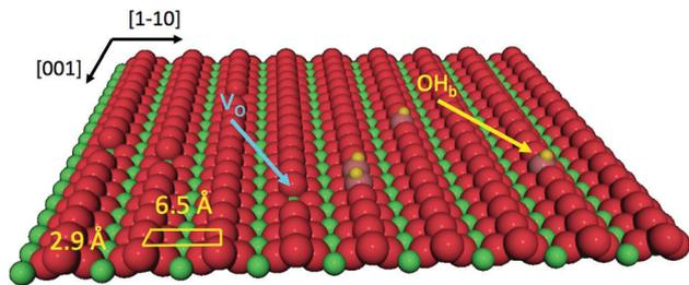
Fig. 1 Perspective view of the  $\text{TiO}_2(110)$  surface termination where oxygen and titanium atoms are represented by red and green spheres, respectively. Point defects, such as oxygen vacancies ( $V_{\text{O}}$ ) and hydroxyls ( $\text{OH}_{\text{b}}$ ), are also indicated.
