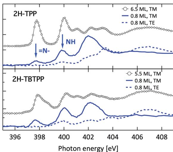
Fig. 6 Nitrogen K-edge NEXAFS spectra of the 2H-TPP and 2H-TBTPP films of Fig. 3 (top and bottom panels, respectively). NEXAFS measurements in TM and TE polarization (full and dashed lines, respectively) are shown for the 0.8 ML films, whereas only spectra in TM polarization are shown for multilayers (open markers).
