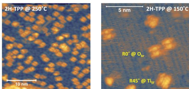
Fig. 20 Left: STM image (PtIr tip) of  $\sim 0.2$  ML 2H-TPP molecules after self-metalation at 250 °C (+1.3 V, 96 pA). Right: A close-up view of isolated TPP molecules after self-metalation at 150 °C (+1.5 V, 40 pA).
