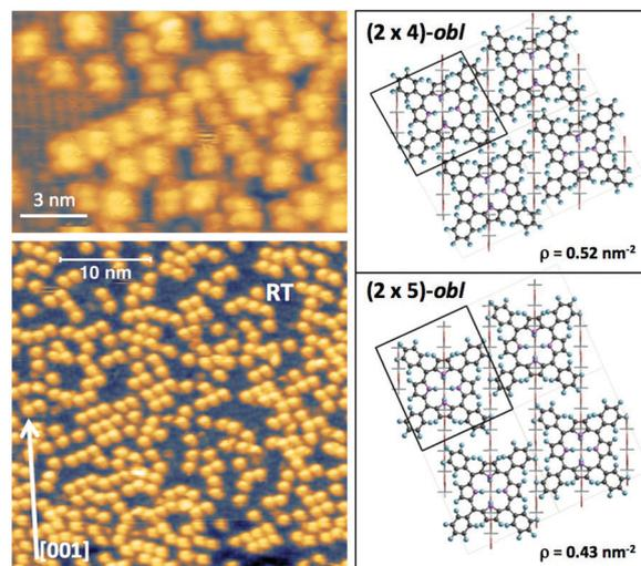
Fig. 12 Left: STM images (Colibri tip) of a  $\sim$ 0.5 ML film of 2H-TTP deposited at RT, where small domains with local  $(2 \times 4)$ -obl order start to form; top and bottom panels correspond to the same film measured at positive (+1.3V, 40 pA) and negative (−1.3V, 140 pA) biases, respectively. Right: Top views of the  $(2 \times 4)$ -obl and  $(2 \times 5)$ -obl phases are shown in the top and bottom panels, respectively.
