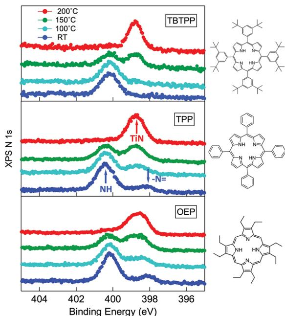
Fig. 10 From top to bottom: the N 1s spectra of 2H-TBTPP (0.8 ML), 2H-TTP (1.1 ML) and 2H-OEP (1.1 ML) as deposited at RT and after annealing; the annealing temperatures are indicated in the top panel; arrows in the central panel (TPP) mark the binding energies of pyrrolic (NH), iminic (=N-) and metalated (TiN) nitrogen. Reproduced from ref. 48 with permission from Elsevier, Copyright 2021.
