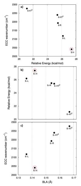
Fig. 5 Correlation between physical quantities sensitive to  $\pi$ -electrons conjugation. Panel a: ECC phonon wavenumber vs.  $\Delta E$  ( $\Delta E$  is the relative crystal energy – per atom – referred to graphene, see text). Panel b:  $\Delta E$  vs. BLA parameter. Panel c: ECC phonon wavenumber vs. BLA. The data corresponding to 6-H crystal is highlighted by a red circle.
