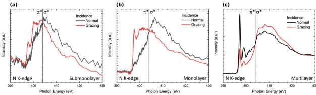
Fig. 5 Nitrogen K-edge NEXAFS spectra measured at normal (E<sub>II</sub> substate) and grazing (E<sub>I</sub> substrate) incidence for different H<sub>2</sub>Pc coverages: (a) subomolayer, (b) monolayer, and (c) multilayer coverages. Sharp features below 404 eV correspond to 1s  $\rightarrow \pi^*$  transitions and a broad feature above 404 eV corresponds to 1s  $\rightarrow \sigma^*$  transitions.
