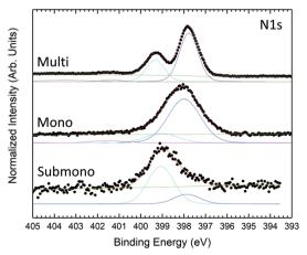
Fig. 3 N 1s core level photoemission spectra measured at 600 eV photon energy for H<sub>2</sub>Pc coverages of one sixth of the monolayer, monolayer, and multilayer.
