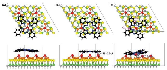
Fig. 7 Optimized configurations obtained for (a) top and (b) bridge positions of H<sub>2</sub>Pc/6H-SiC(0001)-(3 × 3), (c) top positioned SiPc/6H-SiC(0001)-(3 × 3). The top panel shows the top view and the bottom panel shows the side view. The molecule is colored as follows: C-black, N-blue, H-white, and Si-red. The substrate is colored as follows: Si adatoms (first layer S1)-red, Si trimers (second layer S2)-orange, Si (third layer S3)-yellow, Si (fourth layer)green, C-grey, and H-white
