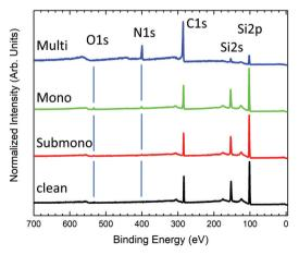
Fig. 1 Photoemission survey measured at 825 eV photon energy for the clean 6H-SiC(0001)-(3  $\times$  3) surface (black curve), one sixth of the  $H_2Pc$ monolayer (submono, red curve), the H<sub>2</sub>Pc monolayer (green curve), and the multilayer (about 20 layers, blue curve).
