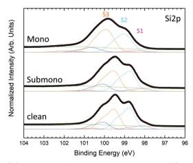
Fig. 4 Si 2p core level photoemission spectra measured at 150 eV photon energy for H<sub>2</sub>Pc coverages of one sixth of the monolayer, the monolayer and the multilayer.
