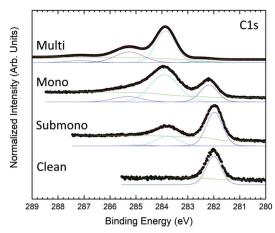
Fig. 2 C 1s core level photoemission spectra measured at 335 eV photon energy for the clean 6H-SiC(0001)-(3 × 3) surface, and H<sub>2</sub>Pc coverages of one sixth of the monolayer and one monolayer and at 485 eV for the H<sub>2</sub>Pc multilayer
