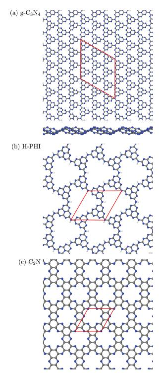
Fig. 1 Periodic single-layer models used for (a)  $g-C_3N_4$ , (3  $\times$  3) cell, top and sideview; (b) H-PHI; (c) C<sub>2</sub>N. Elementary cells in red, C in grey, N in blue H in white
