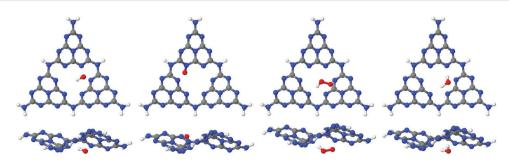
Fig. 3 Adsorption of OH, O and OOH (the products of reactions A, B and C in the OER), and of H<sub>2</sub>O, on a single-pore cluster model of g-C<sub>3</sub>N<sub>4</sub>, NH<sub>2</sub>saturated. Shown are the topviews (upper panels) and sideviews (lower panels) of the single-layer models. All structures calculated based on periodic PBE+D3 starting structures of ref. 16, then a constrained reoptimization on the PBE+D3/6-311G\*\* level of theory was performed as described in the text.
