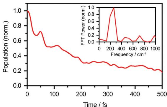
Fig. 6 Calculated population dynamics of aqueous  $\text{PhOH}^{\bullet+}$ , obtained from *ab initio* quantum dynamics simulations. The population decays to a  $1/e$  value in 193 fs. The inset shows the FFT power spectrum, which reveals an oscillatory frequency of  $229 \text{ cm}^{-1}$ .
