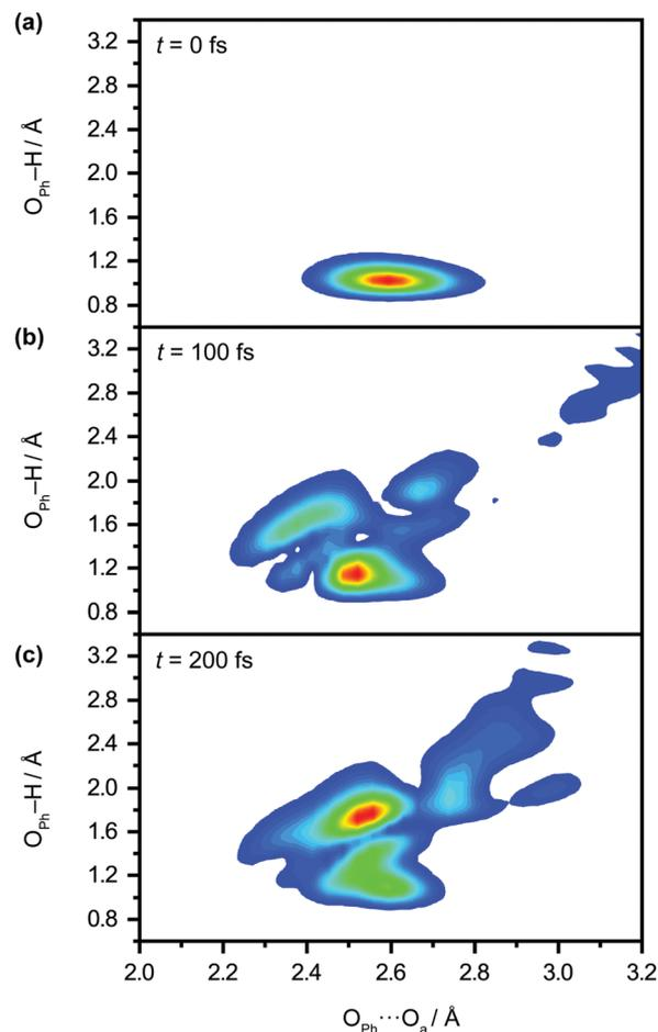
Fig. 5 Quantum dynamics simulations of proton transfer in aqueous  $\text{PhOH}^{*\dagger}$  yields the time-dependent vibrational probability density at time delays of (a) 0 fs, (b) 100 fs, and (c) 200 fs.
