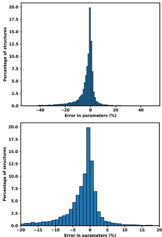
Fig. 1 Error in cell parameters, calculated as  $(X_{\text{GFN}} - X_{\text{Exp}})$  (a–c). Right hand side shows the 95.13% of cell parameters within  $\pm 20\%$  of the experimental value.
