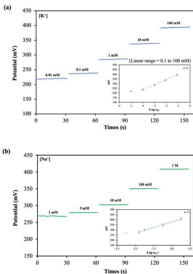
Fig. 3 Potentiometric responses of (a)  $K^+$ -ISE and (b)  $Na^+$ -ISE to varying activity of  $K^+$  and  $Na^+$  ions, respectively. The inset shows a linear relationship between the potential and the logarithm of (a)  $K^+$  and (b)  $Na^+$  activity in 0.1 M HEPES buffer pH 7.4 ( $n = 4$ ).
