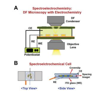
Fig. 2 (A) A schematic showing the experimental setup of the DF microscopy coupled with an electrochemical workstation. (B) Spectroelectrochemical cell diagram with ITO-coated glass as the working electrode (WE), Pt wire CE, insulated Pt guasi-reference electrode (RE), and spacing imager.
