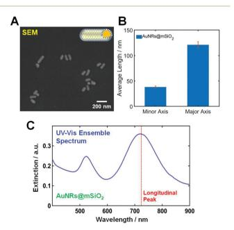
Fig. 1 (A) SEM image of AuNRs@mSiO<sub>2</sub>. (B) Histogram showing the size distribution of AuNRs@mSiO2. (C) UV-Vis extinction spectrum of AuNRs@mSiO<sub>2</sub>. The red-dotted line indicates the position of the longitudinal LSPR peak.
