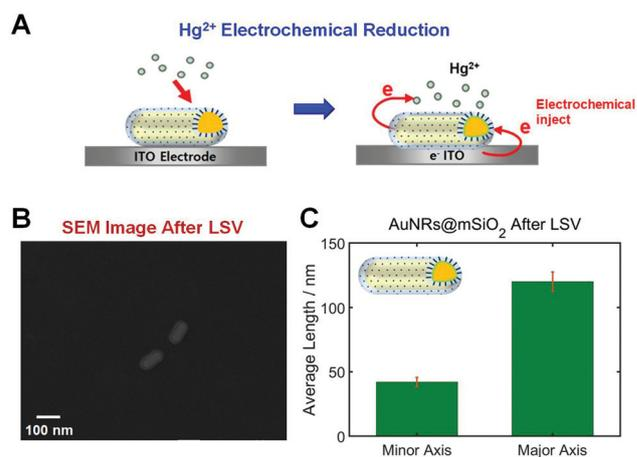
Fig. 3 (A) Schematic depiction of Hg<sup>2+</sup> electrochemical reduction occurring on the AuNR core inside the mesoporous silica shell on an ITO glass. (B) SEM image of AuNRs@mSiO<sub>2</sub> after LSV in the presence of 10 μM HgCl<sub>2</sub>. (C) Histogram showing the change in the sizes (length and width) of AuNRs@mSiO<sub>2</sub> after LSV and Hg amalgamation.
