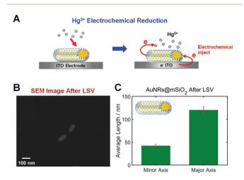
Fig. 3 (A) Schematic depiction of Hg2+ electrochemical reduction occurring on the AuNR core inside the mesoporous silica shell on an ITO glass. (B) SEM image of AuNRs@mSiO2 after LSV in the presence of 10 μM HgCl<sub>2</sub>. (C) Histogram showing the change in the sizes (length and width) of AuNRs@mSiO2 after LSV and Hg amalgamation.
