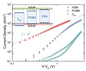
Fig. 11 Current density vs. voltage characteristics of ICBA (213 nm), [60]PCBM (222 nm), and  $C_{60}$  (227 nm) hole-only devices, corrected for the built-in voltage ( $V_{bi}$ ). The grey dashed line indicates a quadratic voltage dependence. The inset shows a schematic energy diagram, indicating the IE and EA of the fullerene derivatives with respect to the trap-free window (dashed lines) (reprinted by permission from Macmillan Publishers Ltd: Nat. Mater., ref. 45, copyright 2019).
