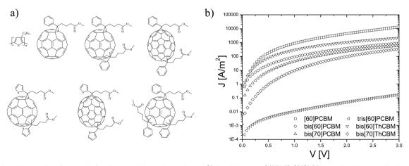
Fig. 7 (a) Materials overview: from top left to bottom right, regioregular poly[3-hexylthiophene] (P3HT), [60]PCBM, and highly generalized structures for the isomeric mixtures of the bisadducts, bis[60]PCBM, bis[70]PCBM, bis[60]ThCBM and bis[70]ThCBM, and the trisadduct tris[60]PCBM. (b) J-V characteristics of the P3HT:fullerene blend electron single carrier devices (reprinted with permission from ref. 31. Copyright 2009 Wiley-VCH Verlag GmbH & Co. KGaA, Weinheim.).
