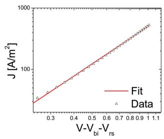
Fig. 6 Current density vs. voltage, corrected for built in voltage and series resistance of a bisPCBM electron only device. Data (symbols) is fitted (solid line) using a space charge limited current with a mobility of  $7\times10^{-8}~\text{m}^2~\text{V}^{-1}~\text{s}^{-1}$  (reprinted with permission from ref. 30. Copyright 2008 Wiley-VCH Verlag GmbH & Co. KGaA, Weinheim).
