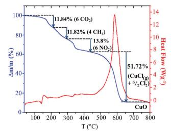
Fig. 5 Simultaneous TGA-DSC curves for the decomposition of the (C<sub>5</sub>H<sub>8</sub>N<sub>3</sub>)2[Cu<sub>2</sub>Cl<sub>6</sub>] cluster.
