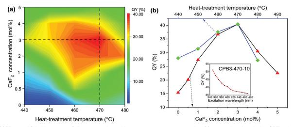
Fig. 4 (a) 2D map of QY with respect to CaF<sub>2</sub> concentration and heat-treatment temperature under 400 nm wavelength excitation. (b) The dependence of the QY on the CaF<sub>2</sub> concentration and heat-treatment temperature. (The inset shows the QY of sample CPB3-470-10 under different excitation wavelengths.)
