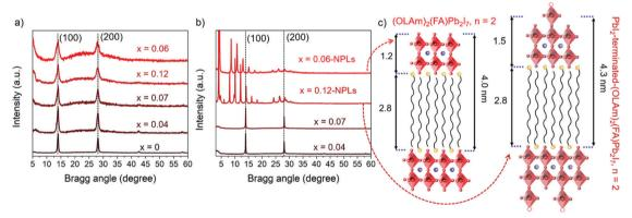
Fig. 2 XRD patterns of the (a) FAPb<sub>1-x</sub>Sr<sub>x</sub>I<sub>3</sub> PQDs colloidal solutions, and (b) their corresponding redispersed precipitates. (c) Schematic representations of the layered perovskite spacings and relevant distances for FAPb<sub>0.88</sub>Sr<sub>0.12</sub>I<sub>3</sub> and FAPb<sub>0.94</sub>Sr<sub>0.06</sub>I<sub>3</sub> NPLs.
