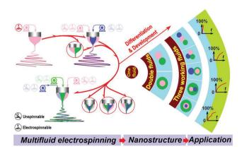
Fig. 4 A schematic diagram showing the possible arrangements of liquids in multi-fluid ES, the nanostructures which can be produced as a result, and the potential drug release profiles
