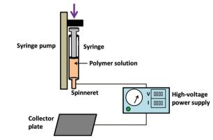
A schematic illustration of the electrospinning process.
