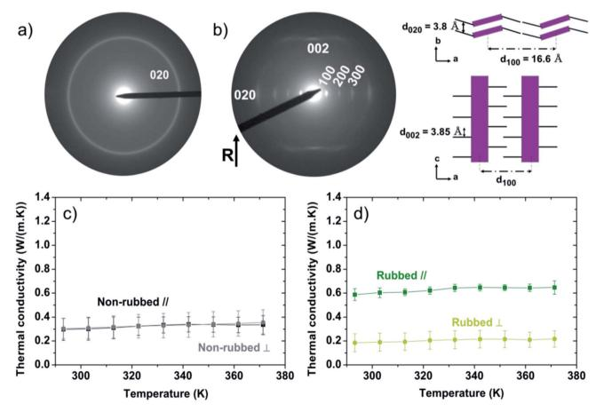
Fig. 2 Electron diffraction patterns of non-rubbed (a) and rubbed P3HT films (b) before doping. The arrow, *R*, indicates the rubbing direction. Schematic of the crystal structure of P3HT (c) and (d) thermal conductivity of non-rubbed P3HT and P3HT rubbed at 171 °C, respectively.
