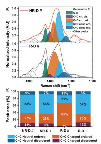
Fig. 4 Raman spectroscopy under 785 nm excitation of the principal molecular vibrations on the thiophene ring: C-C stretching, C=C charged (dis)ordered, C=C neutral (dis)ordered, (a) isotropic doped (NR-D) and rubbed doped (R-D) P3HT along the deposition direction, and (b) total integrated peak area of the four vibration modes of C=C ring breathing for isotropic doped and rubbed doped P3HT in both directions.
