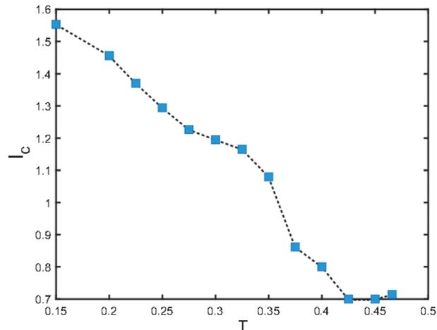
Fig. 4 Critical length scale. We define a length scale,  $l_c$ , given by  $l_c = (t_x - t_\alpha)U_c$  where  $U_c$  is the probe velocity at which we obtained a stationary to non-stationary transition. In liquid phase,  $l_c$  is almost zero, however, near  $T_{mc} = 0.36875$  it has a sharp increase, and then it monotonically increases by lowering the temperature.
