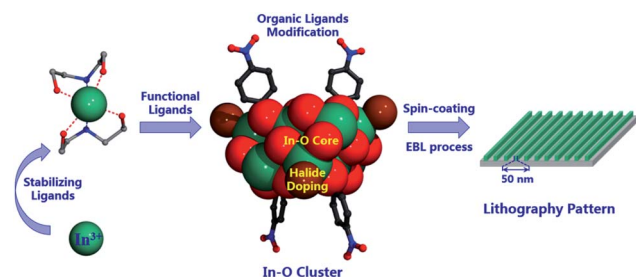
Scheme 1 Illustration of the assembly of the atomically precise \text{In}_{12} -oxo clusters with chemical modification and patterning evaluation.
