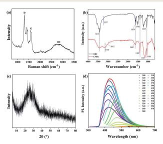
Fig. 5 (a) Raman spectrum, (b) FT-IR spectra, (c) XRD and (d) corresponding PL spectra at different excitation wavelengths from 300 nm to 580 nm for CNDs.
