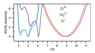
Fig. 4 Free energy as a function of coordination number of  $Cr^{3+}$ ,  $Mg^{2+}$ , and  $K^+$ . Solid and dashed lines indicate the KCl-MgCl<sub>2</sub> salt mixtures with and without  $Cr^{3+}$ , respectively.
