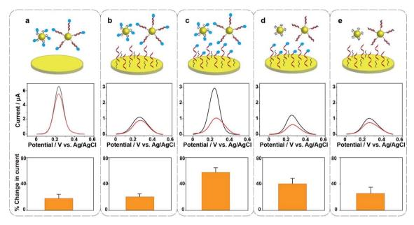
Fig. 2 Hybridization-induced change in background-subtracted SWVs and percentage change in current after exposing the sensor to 20 nM complementary target DNA (22 nucleotides) in five different systems as indicated by the cartoons. Electrolyte solution was 0.5 mM  $K_3$ [Fe(CN)<sub>6</sub>] in phosphate buffered saline (pH 7.4). The frequency and pulse amplitude of SWVs were 2 Hz and 25 mV, respectively. Error bars represent standard deviations from at least 3 independent measurements.
