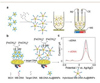
Fig. 1 Schematic illustration of DNA-mediated reduction of potassium ferricyanide (K<sub>3</sub>[Fe(CN)<sub>6</sub>]) by methylene blue (MB). (a) Workflow for the measurement of target ctDNA. (b) Electrochemical sensing mechanism of the DNA sensor. (c) Background-subtracted square wave voltammograms (SWVs) in the absence and presence of target ctDNA (101 nucleotides). The frequency and pulse amplitude of square wave voltammograms were 2 Hz and 25 mV, respectively.
